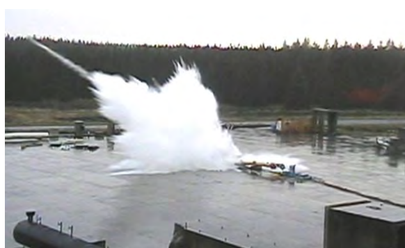
Fountain. Underwater burst tests show weak spots.
