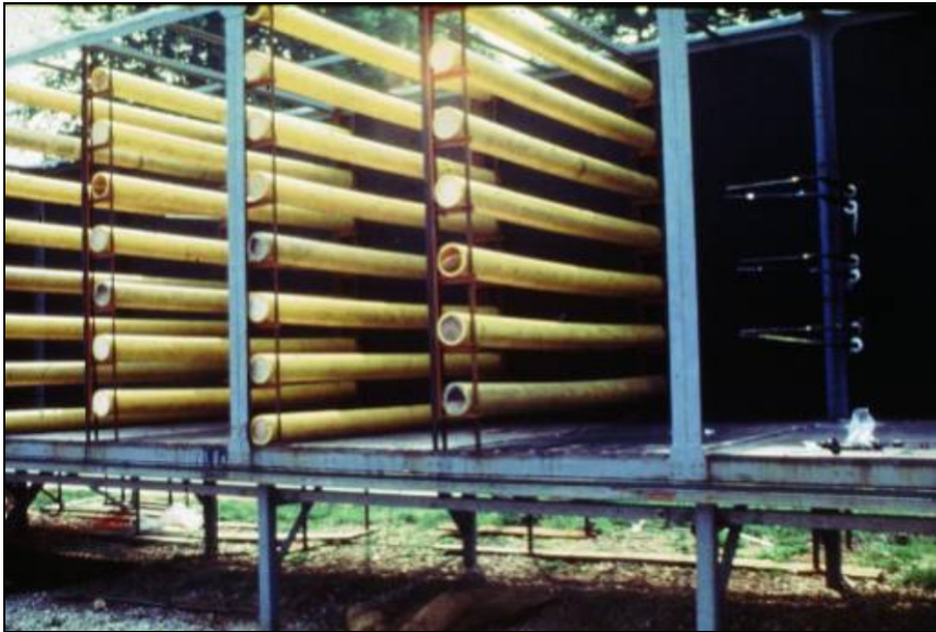
Figure 4: Obstacle Configuration Used in 45m Long Test Rig
