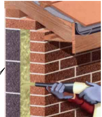
Cavity wall insulation
